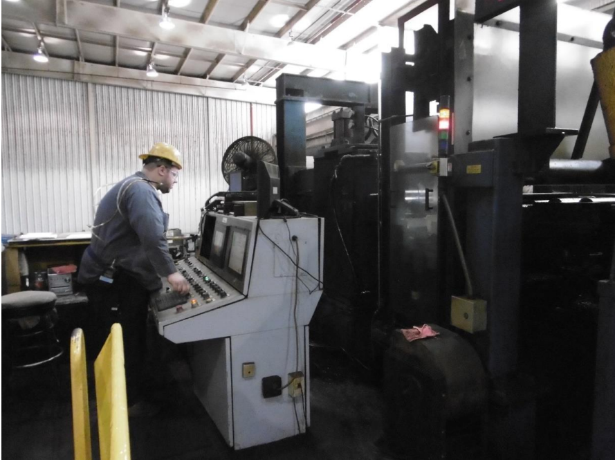
Exit operator at station controlling electrostatic oiler. Photo by NIOSH.
