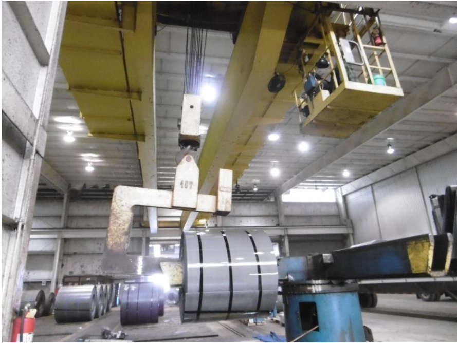
Steel coil after pickling process. The rust has been removed and additional oil is rolled on the outside to protect the steel. Photo by NIOSH.
