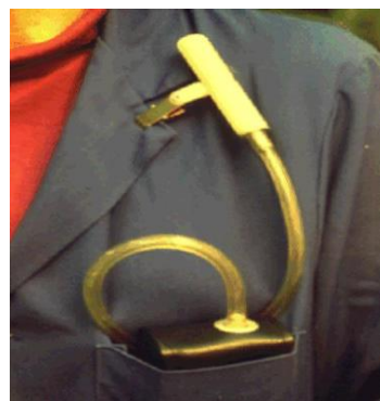
Figure 9.3 – Personal Sampling With Sorbent Tube Collection
