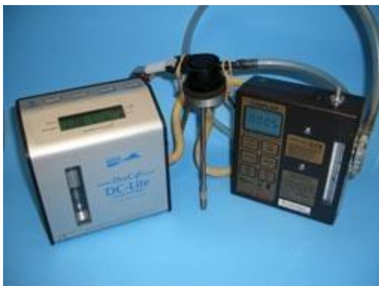
Figure 8.21 – Calibration Using an Electronic Meter
