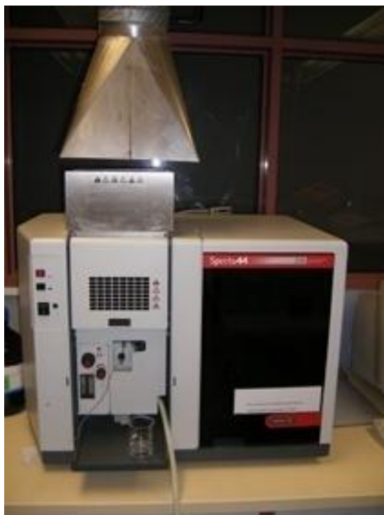
Figure 7.1 – Schematic of an Atomic-Absorption Spectrometer
