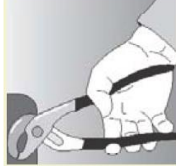
Figure 4.17 – Repetitive movements of the fingers is required to open pliers because the tool has no return spring. Repetitive use of pliers requires awkward movements and postures of the hands
