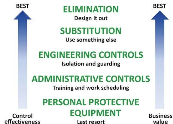
**Fig. 2** Prevention through Design using hierarchy of controls (Peterson 1973)
