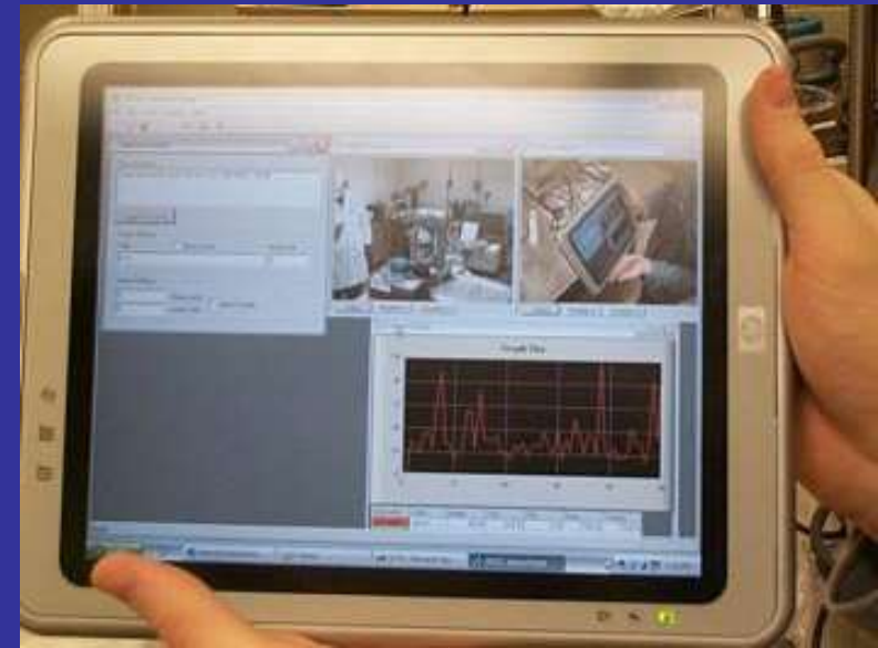
Integrated VEM with real-time sensor output and data logging
